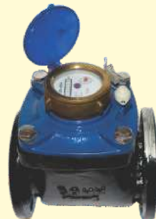
A removable mechanism type Woltmann water meter with magnetic drive and vacuum sealed register.
